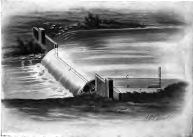
FIG. 9. —Gauging the Discharge of a Stream.
